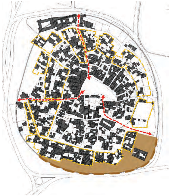
Figure 8. Continuous blocks to the south and south-east limit sand from dune encroachment
