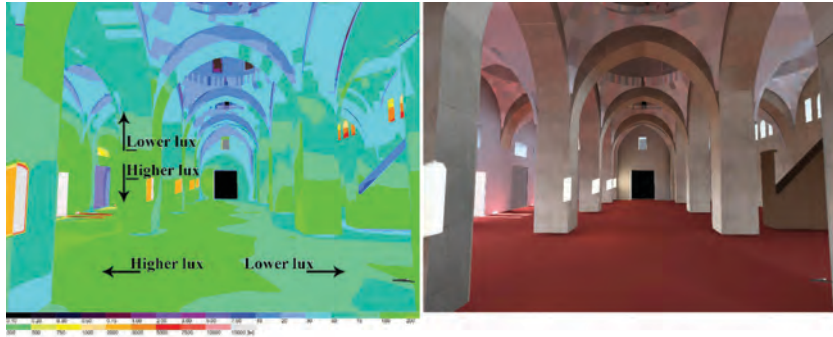
Figure (12): Vertical and horizontal gradient of illuminance level (E) created contrast between the entrance zone and Minbar zone, as well through in the vast height of the structure. (Al-’Aṣr, winter, clear sky).
