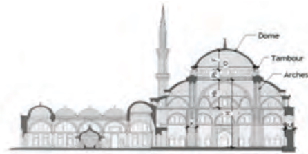
Fig: Different entities of Ottoman Mosque: Sectional View.
